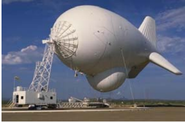
Figure 8: Current-generation aerostat - Tethers Aerostat Radar System (TARS) from ITT Systems Division.
