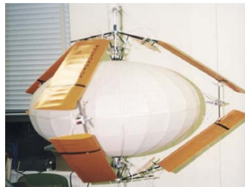
Figure 9: 4 ft. diameter scale model of the VectoRotor used for static and indoor free flight tests.
